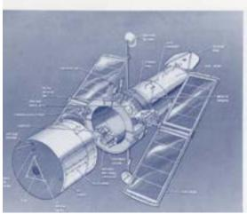
SUPPORT SYSTEMS MODULE — Overall size of the Space Telescope is 43 feet (13.1 meters) long by 14 feet (4.26 meters) in diameter. This illustration shows the Support Systems Module, which contains the very precise pointing and stabilization control system, communications, thermal control, data management and electric power systems, and solar panels for electrical power generation.
